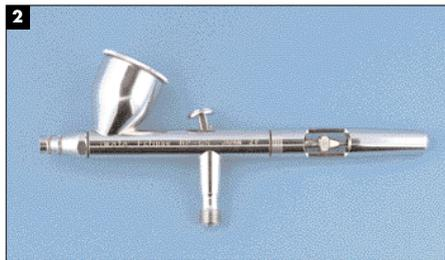
This is an Iwata Eclipse series double-action airbrush. Pressing down on the top button turns on the air flow; rocking the button back and forth controls the paint volume. This model has a gravity feed paint cup.
