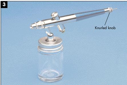
Badger's model 200 is a hybrid design. It has the longitudinal needle found on double-action airbrushes, but the paint volume is controlled by turning the knurled knob at the end of the needle.
