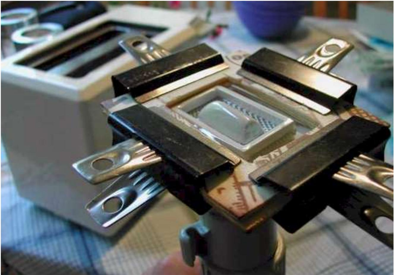
A new canopy, which turned out to be less than excellent. More polishing of the plug needed!
