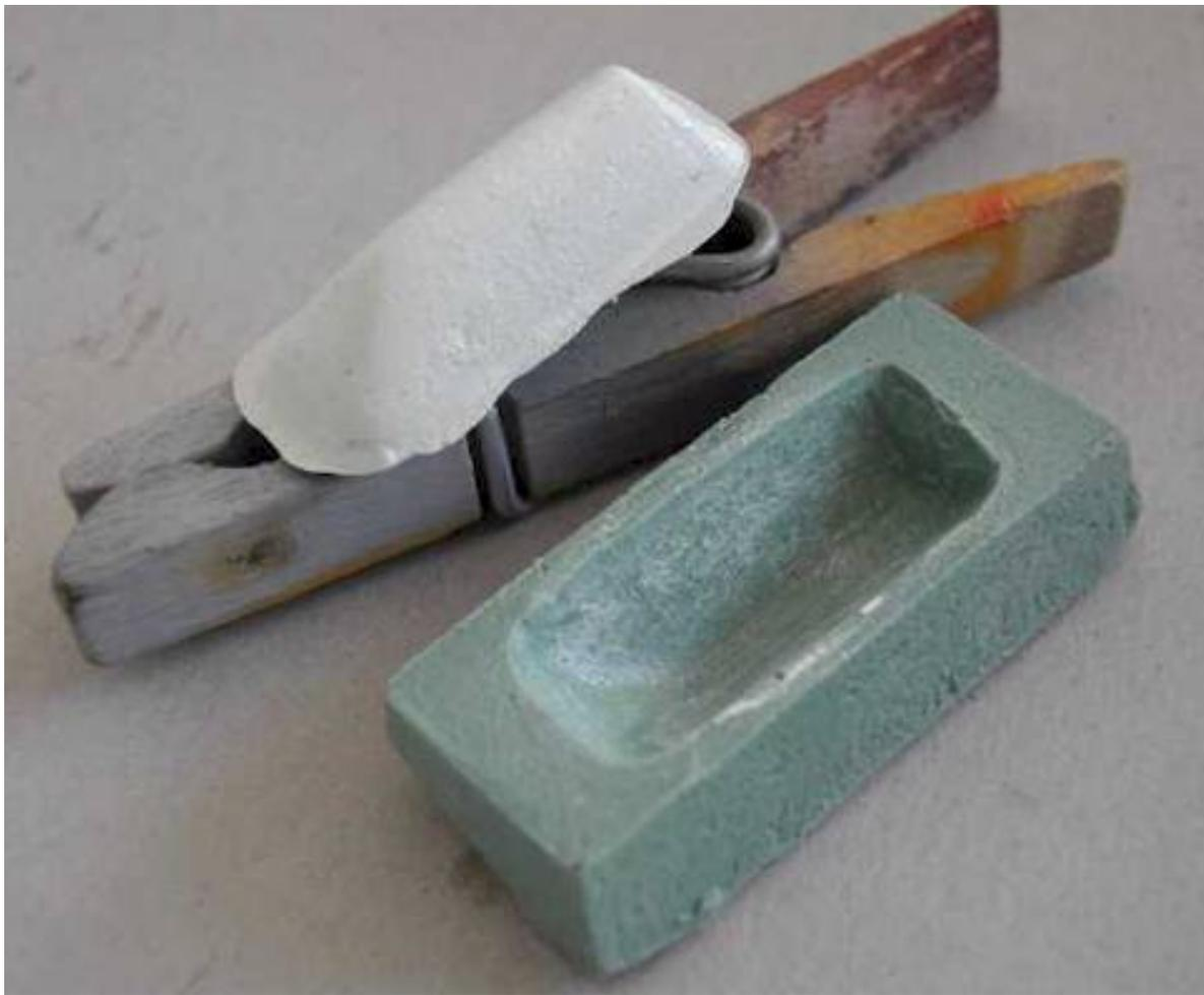
The Milliput plug fresh from the mould. It will be sanded and covered in a thin layer of CA glue and then polished
