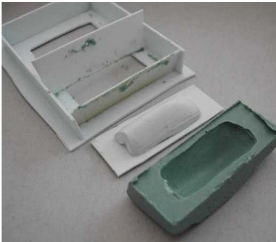
The Plastic Padding mould which then is used to cast another Milliput plug. This will then be sanded and polished to a high-gloss finish so that a new canopy can be vac-formed over it.
