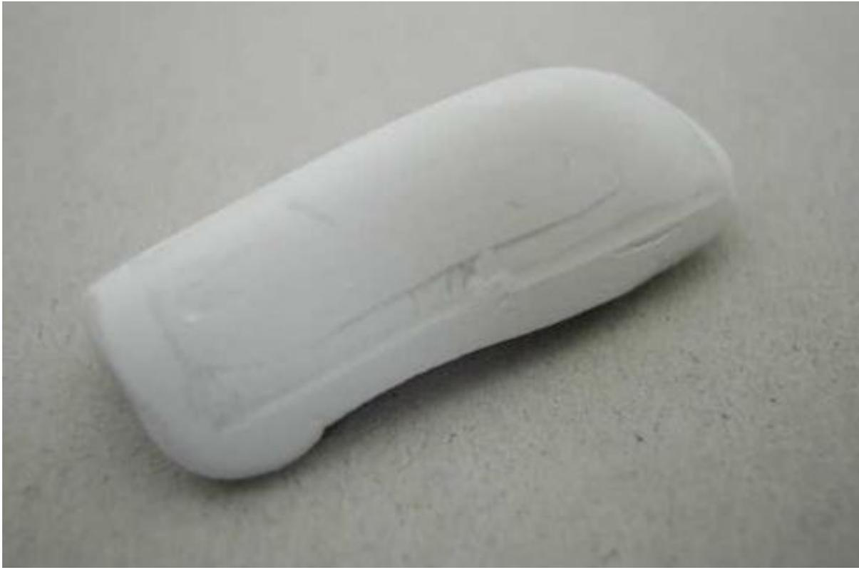
This is the original Marivox kit canopy, filled with Milliput and sanded down so as to make it slightly smaller than the original. No polishing needed at this stage!
