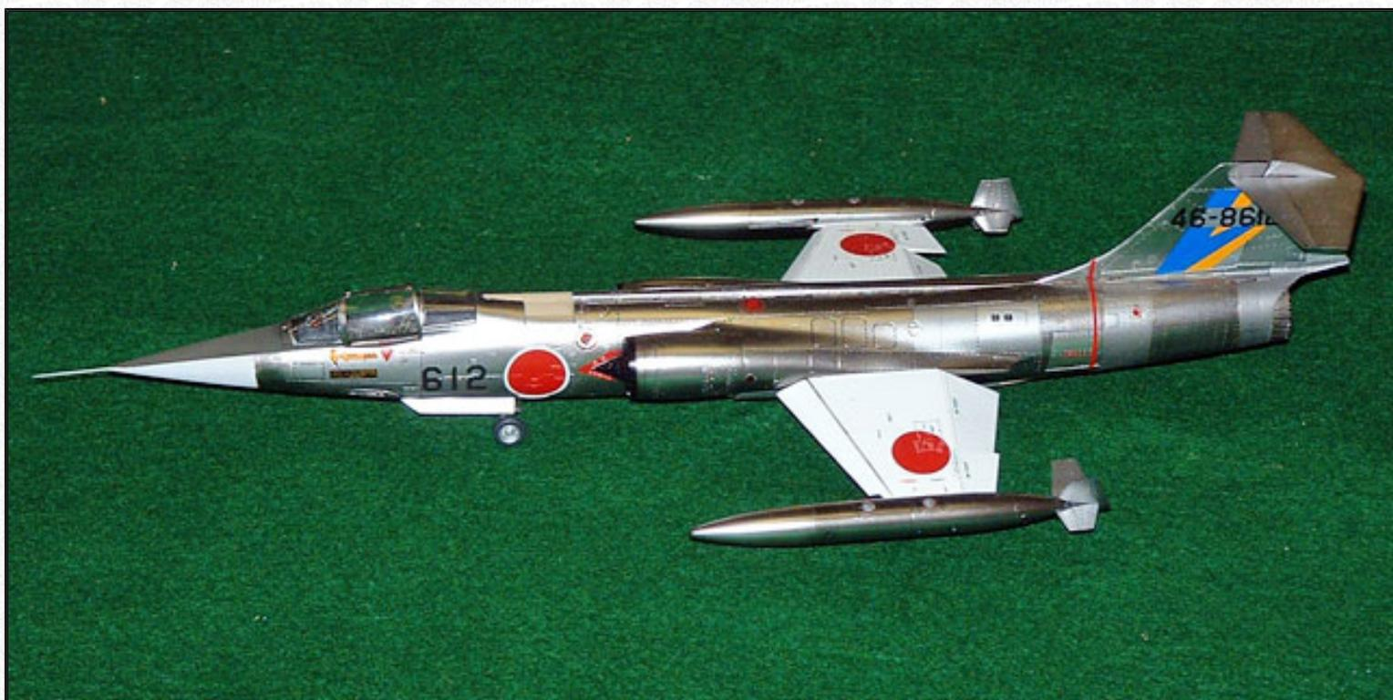
Figure 5: The author's Hasegawa F-104J painted with Alclad II Chrome as the base coat and varying shades of Alclad II and Testor's Metalizer for individual panel areas.
