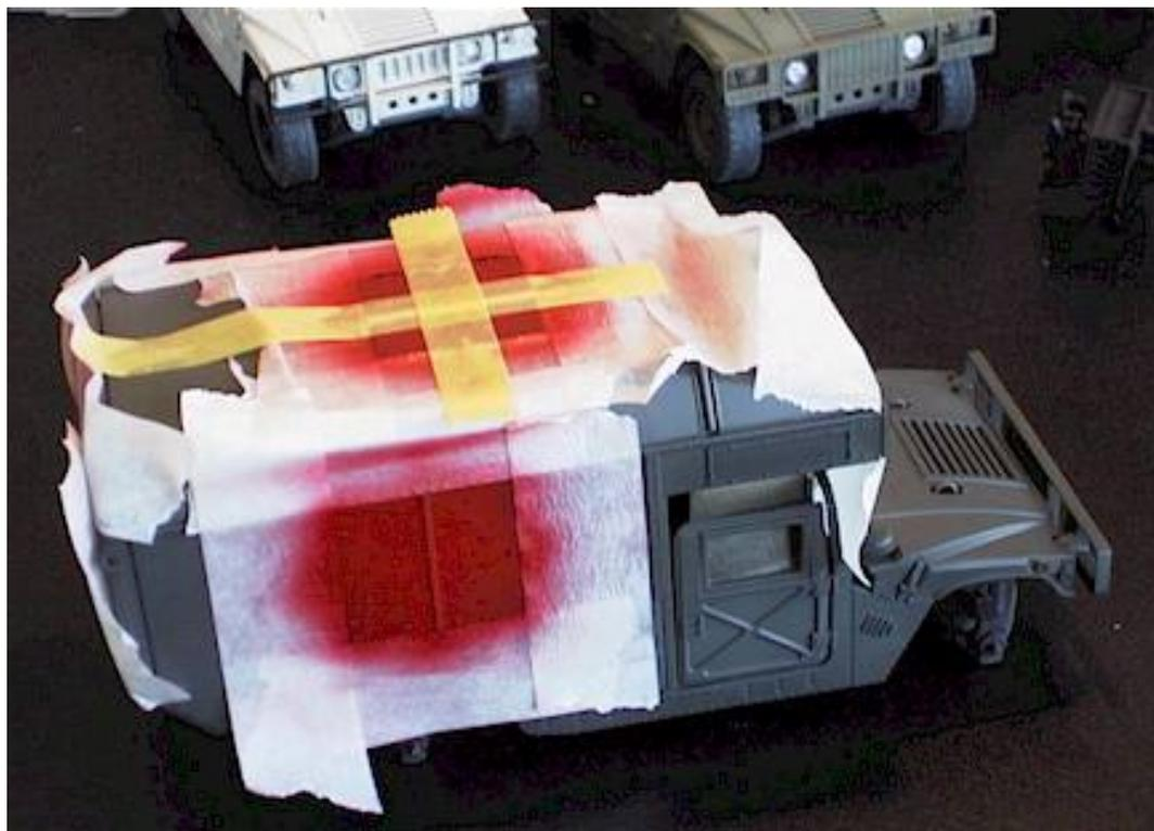
The sequence of masking and painting is shown on the picture to the left. First, the entire square area of the red cross marking has been masked (white tape, see the side of the vehicle).
