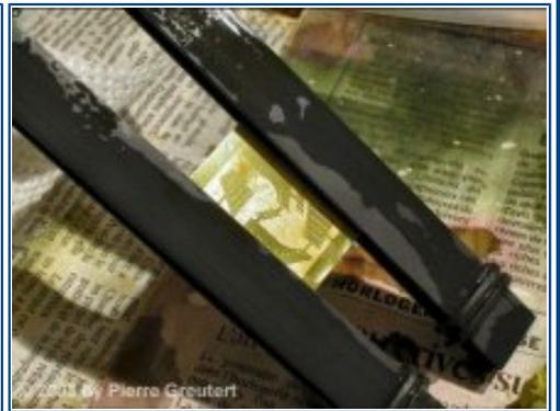
Well, the etching is almost finished, and everything went well. The Scale PhantomPhixer is happy! Time now to strip away the photoresist that protected the parts. Isopropyl alcohol is fine for the job. The piece is now somewhat dull, so a last bath in a solution of vinegar + salt turns it into a shining beauty.
