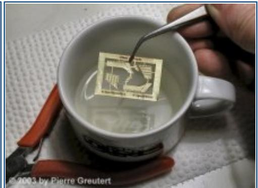
Et voilà! You might wonder how I engraved the text on the border? Remember that the etching fluid will eat brass from both sides. Since the text is only printed on the top transparent - not on the back - the etch will be only half way through when areas which are transparent on both sides are fully through. This is the way to etch folding lines, engraved or embossed panels, rivets, etc
