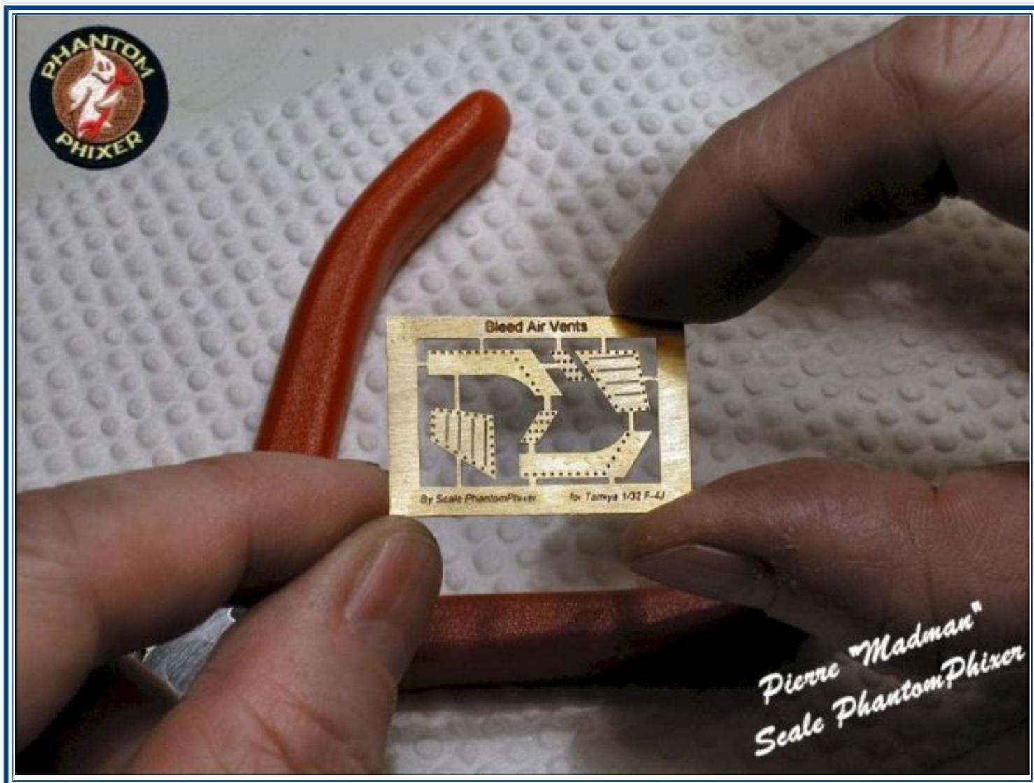
Here is the vent, cut away from the brass sheet. The vent area on the fuselage gets a coat of filler to mask the mishaps. I fold the vent blinds, by twisting delicately each blind with a surgeon scalpel. The filler can dry during this time, and it is now ready to be sanded smooth. In the middle of the vent area, I want to make some room for the blinds, and to simulate the exit duct.
