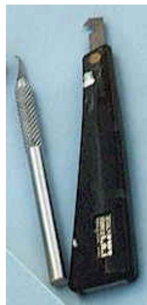
A pointed (e.g., No. 11 X-Acto) knife blade held in a slender handle also is helpful in some situations, because the tip of such a blade can be manipulated very precisely. However, a knife blade's disadvantages are that it tends to wander along the path of least resistance through a plastic surface, and it tends to cut too deeply. In situations where a pointed knife blade seems best, I either use the *back* (rather than the sharpened) side of the blade tip, or I
